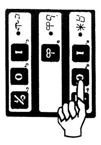
1 • Push on key a to stop the cooling function.
