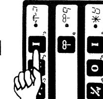
5 • Push on key c<sub>1</sub> to start the automatic cleaning.
