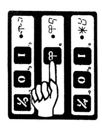
2 • For sampling, push on key b for a 2 min. agitation.
