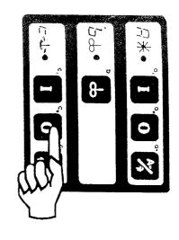
1 • Push on key c<sub>o</sub> to stop the cleaning function.
